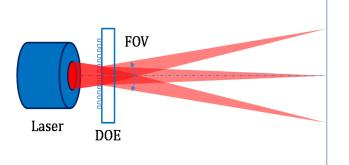
A DOE functions with a laser light source that emits a diffractive pattern. Each DOE pattern is characterized by a specific laser wavelength, focal length and transverse mode. Each laser wavelength will result in a different zero order intensity. The focal length is dependent on the DOE and the object distance which can be adjusted using a collimating lens (CL). The transverse mode will affect the dot shape.
